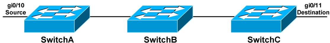
The SPAN source exists on SwitchA, and the SPAN destination exists on SwitchC. Each switch must be configured with the RSPAN VLAN, including the intermediary SwitchB.
